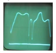
Figure 2: Splitting of the central mode of the Bragg resonator (cold measurements)
