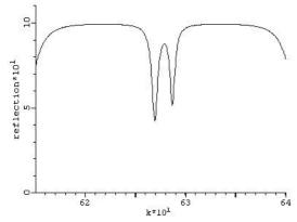
Figure 3: Splitting of the central mode of the Bragg resonator (numerical simulation)
