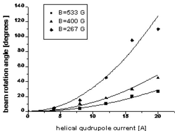
Figure 3: Dependence of the beam rotation angle on the helical quadrupole current at different longitudinal magnetic fields
