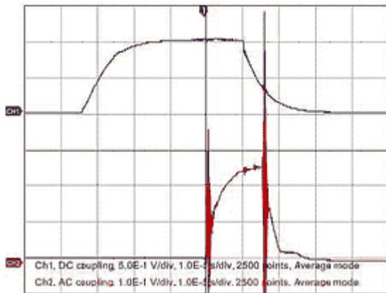
Figure 7: Time dependence of kicker signal (top curve) and pulse of injected electron beam (bottom curve). Time scale: 10 μs/div
