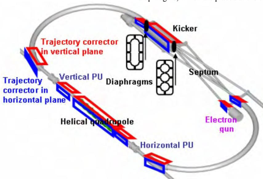
Figure 5: Beam diagnostic tools and correction coils disposition
