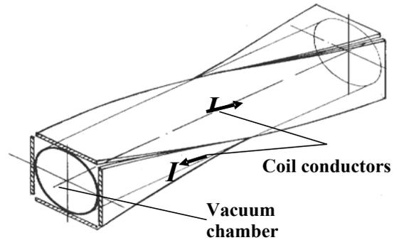
Figure 2: Scheme of the helical quadrupole
