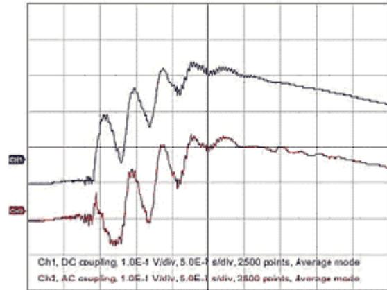
Figure 8: A few first turns of the beam in the ring. Signals from vertical PU station
