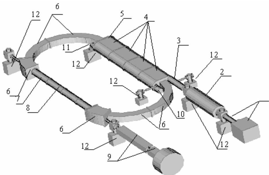
Figure 1: Design of the LEPTA. 1 – positron source, 2 – positron trap, 3 – positron transfer section, 4 – septum solenoids, 5 – kicker (inside septum solenoid), 6 – toroidal solenoids, 7 – solenoid and helical quadrupole inside it, 8 – electron cooling section, straight solenoid, 9 – experimental channel, 10 – electron gun, 11 – collector of the electrons, 12 – vacuum pumps
