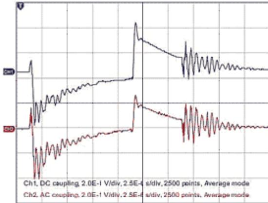
Figure 6: Signals from vertical PU station. Time scale: 2,5 μs/div. Top curve is signal from top plate of the PU station and bottom curve – from bottom plate
