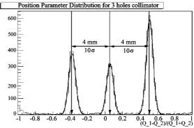
Fig. 7: Results of space resolution test of silicon PSD detector with alpha particles and three-hole collimator.
