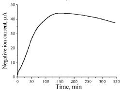
Fig. 3: Time dependence of the output negative ions current from the sputter source.
