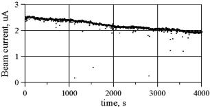
Fig. 4: Time dependence of C - current from gas source in experiment.
