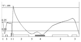
Fig 6: RMS beam size in AMS tract (calculations for  $W_0 = 15 \text{ keV} - \text{initial energy}$ ,  $U_T = 1 \text{ MV} - \text{terminal voltage}$ ), 1 - electrostatic lens, 2 - accelerating tube, 3 - double-focusing magnet,  $4 - 180^\circ$  combined bend, 5 - place of magnesium stripper.
