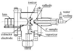
Fig. 2: Scheme of the sputter negative ions source.
