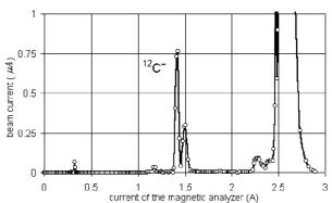
Fig. 5: Typical mass-spectrogram of negative ion beam from gas ion source (on CO<sub>2</sub> gas).
