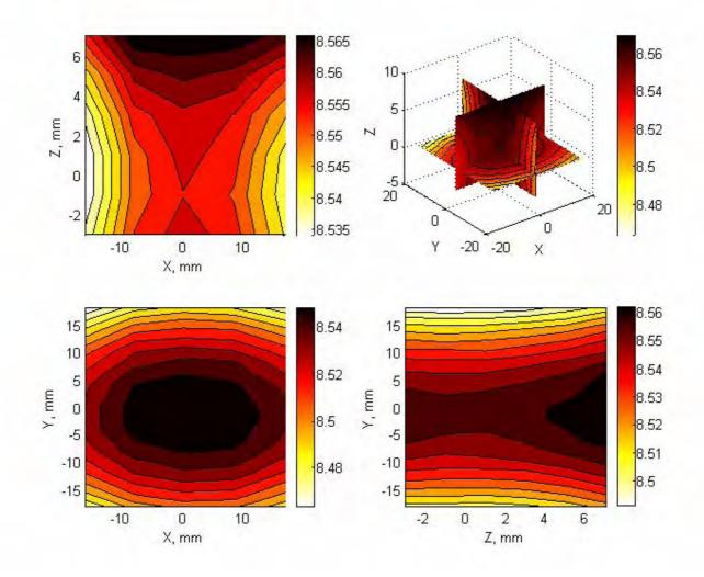
Figure 6: Ddistributions of magnetic field in the center of magnet for working field value 8.5 T.
