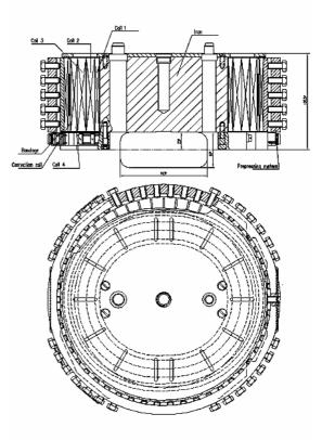
Figure 1: Sketch of assembled coil.
