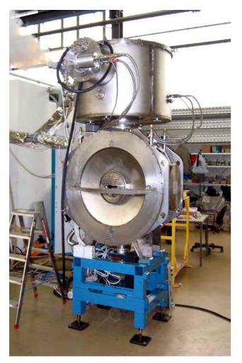
Figure 4: Photo of assembled Superbend cryostat.
