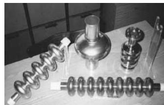
Fig. 3: The copper shells manufactured in the Lab
