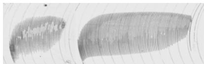
Fig.1: Pocket oscillation under Nb electrochemical polishing
