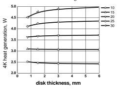
Figure 5: Heat flow to the 5 K heat sink for the design with bellows bi-sectioned
