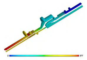
Figure 7: Temperature map of the coaxial part
