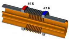
Figure 2: Model of a regular cold bellows
