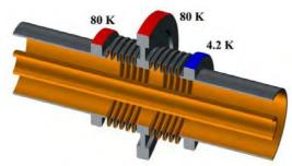
Figure 4: Cold bellows model with an additional 80 K heat sink
