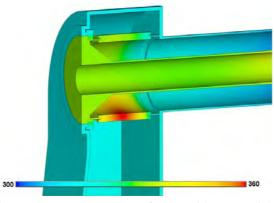
Figure 8: Temperature map of waveguide-to-coaxial transitio
