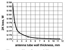
Figure 6: Heat flow to 2 K zone
