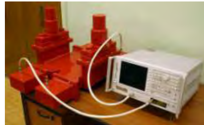
Figure 8: Directional couplers measurement setup
