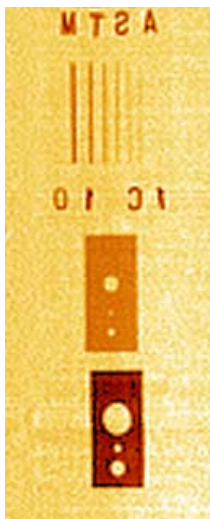
Figure 3: Wire and plate defectometers behind the 200 mm steel barriers
