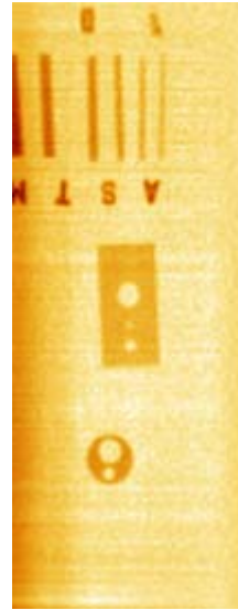
Figure 4: Wire and plate defectometers behind the 300 mm steel barrier
