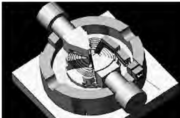
Figure 1: Cyclotron with the Upper Part of the Magnet Removed.
