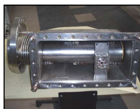
Figure 3: Station of ES beam-pickups, contents of the assembly box (left) and view along beam axis (right).
