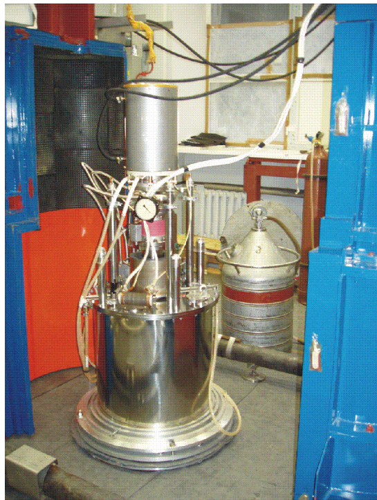
Fig. 3. Photo of the upper part of the stand. Visible components: cryomagnet, calorimeter, part of the biologic protection.
