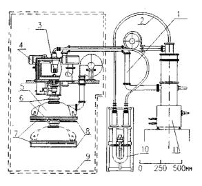
Figure 1: ILU-8 accelerator in local radiation shield.
