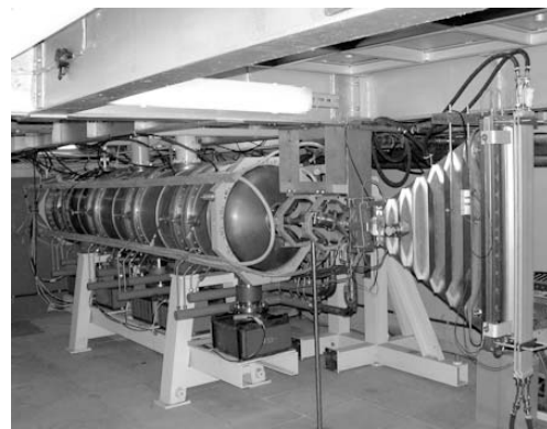
Figure 4: Accelerating structure with beam scanning system.
