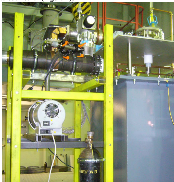
Figure 4: Linac assembly and the modulator.
