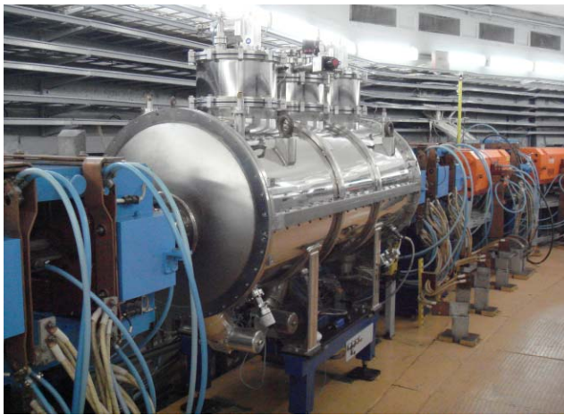
Figure 1: Superconducting wiggler on SIBERIA-2 storage ring.
