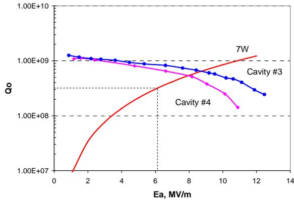
Fig.3. RF characterization results for prototype cavities
