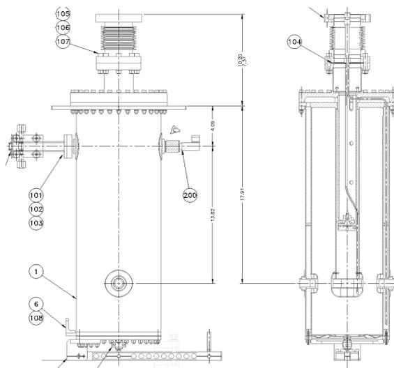
Fig.1. ISAC-II high beta cavity design.
