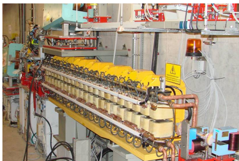
Fig. 3 FLASH far infrared undulator constructed by JINR.
