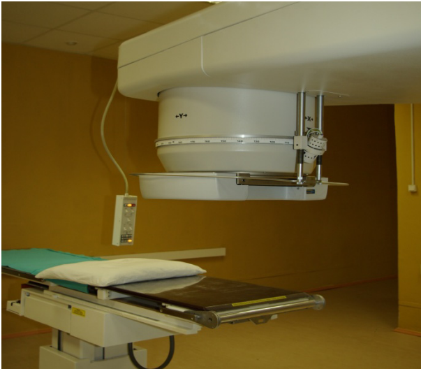
Figure 2: Multileaf collimator mounted on the SL-75-5 accelerator
