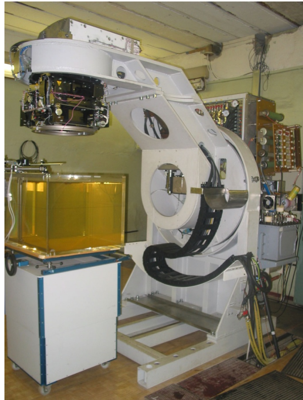
Figure 1: The “ELLUS-6M” accelerator under technical tests; dose fields are being measured in a water phantom
