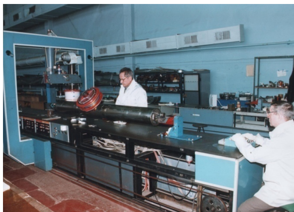
Figure 2: Machine for 6 m length SC coil winding.
