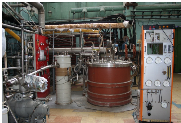
Figure 4: Test facility for study of 1 m length SC magnets. 180 l/h boiling helium.
