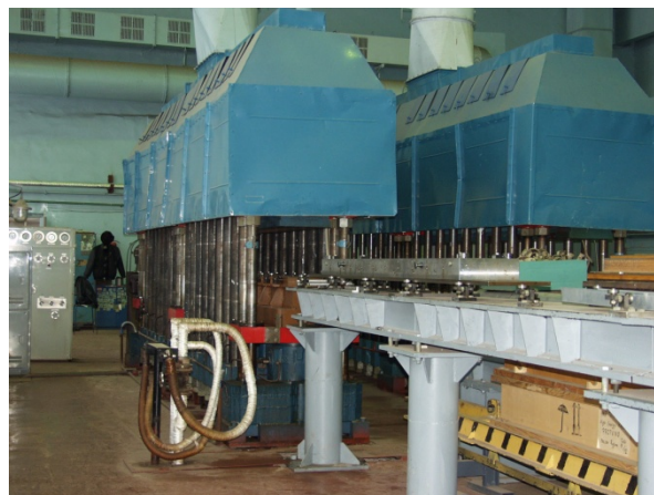
Figure 3: Presses for collaring and curing of SC coil. 3800 tons, L = 7 m, h = 0.67 m.
