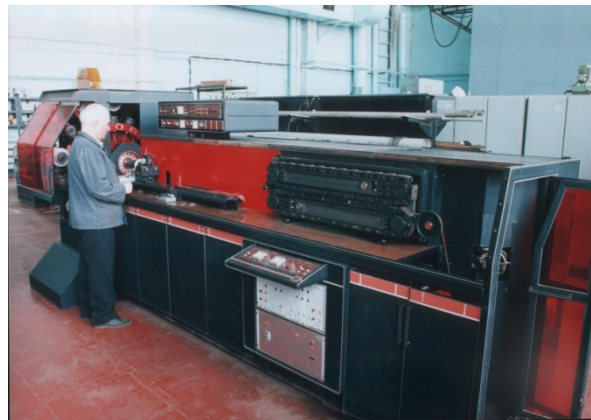
Figure 1: Machine for SC cable production. N_{max}=28 strands of 0.3-1 mm diameter, V=1.5 m/min.
