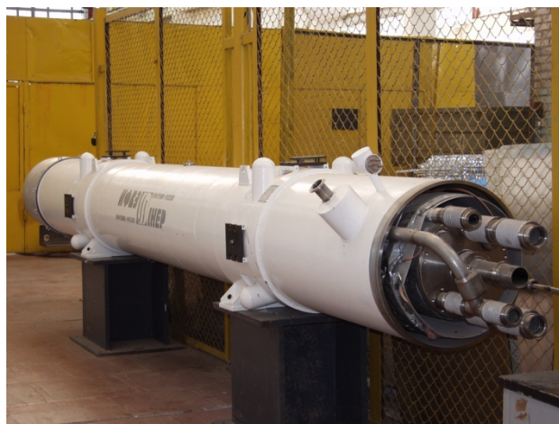
Figure 6: UNK SC dipole magnet.
