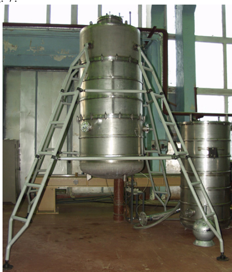
Figure 7: Cryogenic helium vacuum heat exchanger. 10g/s helium flow, 300-2 K temperature range.
