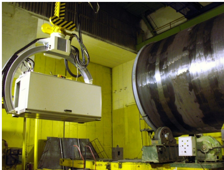
Figure 1: The UEL-10-D accelerator in a shop of the “Izhorskie Zavody” open joint stock company
