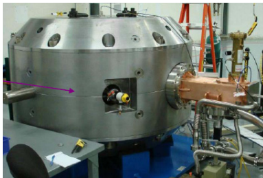
Fig.3. Superconducting Synchrocyclotron with 9 T field built by “Still River”. Weight is 20 tons. [14].
