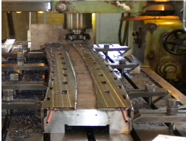
Figure 6: View of the Booster magnet yoke during processing on the milling machine.
