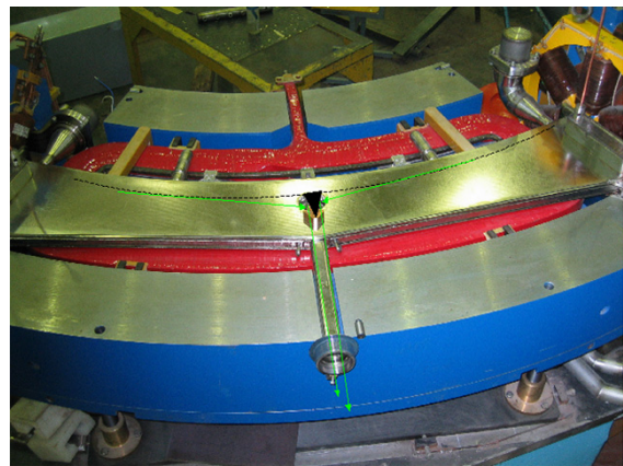
(b) Vacuum chamber and mirror after assembling. Additional mirror is placed in the center for comparison.
