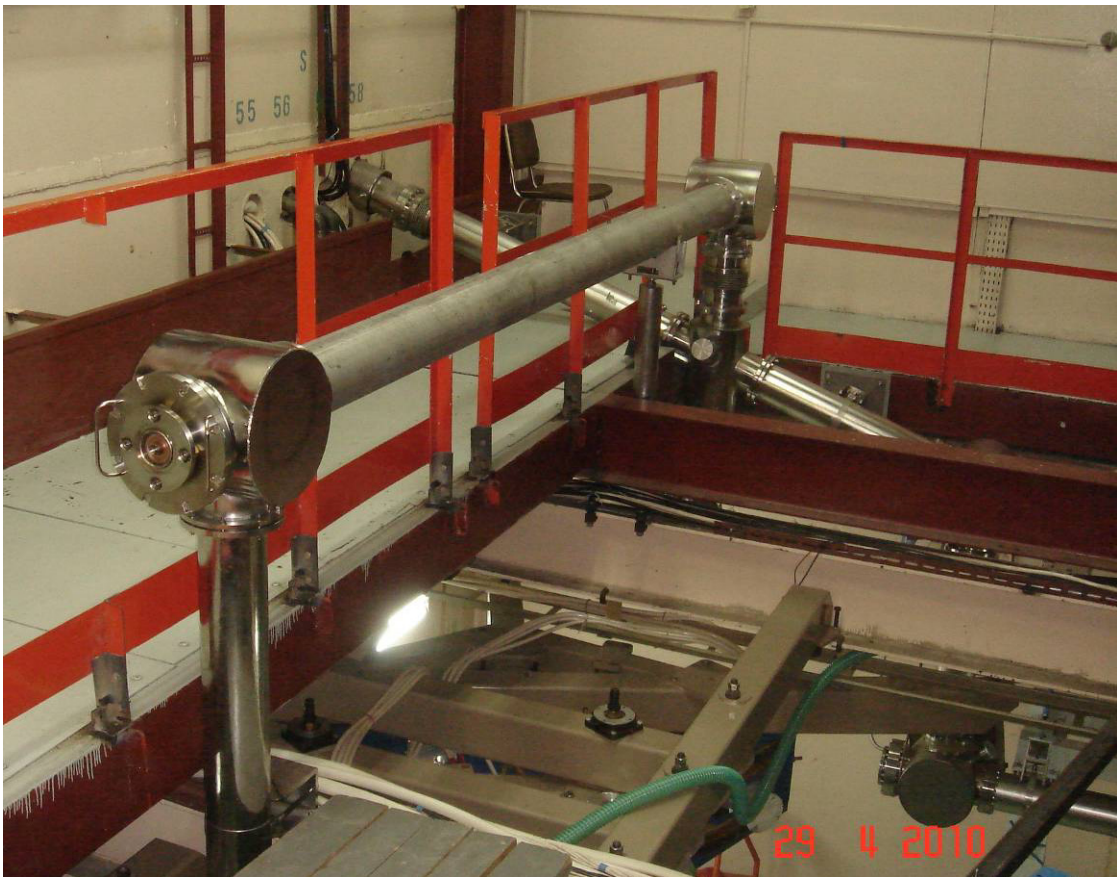
Figure 4: The optical beamline which transport the radiation of the second FEL to the user stations.
