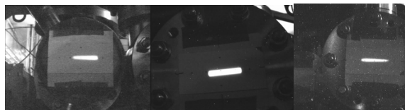
Figure 5: X-Ray beam from 7.5T SCW at output of three beam lines in the experimental hall of Siberia-2.
