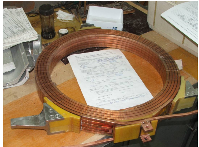
Fig. 4 Coils for the cooling section
