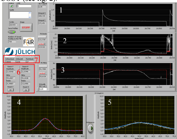
Figure 2: Display of the IPM data acquisition program. Beam Current Transformer (BCT) signal plotted over time (1); horizontal and vertical profile width (Gaussian standard deviation) (2); horizontal and vertical beam position (3); measured vertical beam profile and the corresponding fit (4); measured horizontal beam profile and the corresponding fit (5); summary of vertical and horizontal fit parameters (6); parameters of the current machine cycle (7). The data displayed in 2 and 3 is derived from the corresponding fits. The horizontal axis in 1, 2, 3 represents measurement points. The data acquisition operates at 24 profiles/s. The horizontal axis in 4 and 5 is calibrated in mm. All fits are Gaussian fits.
