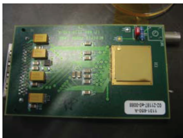
Figure 7: Spectrometric detector on basis of GaAs (Cr) pixel sensor with 256x256 channels of 50 \mu\text{m} resolution and Medipix chip.
