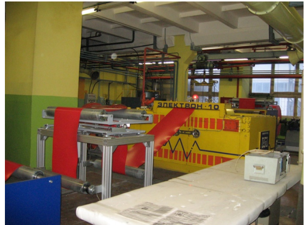
Figure 3: The “Electron-10” accelerator at the Izhevsk Plastic-Production Plant
