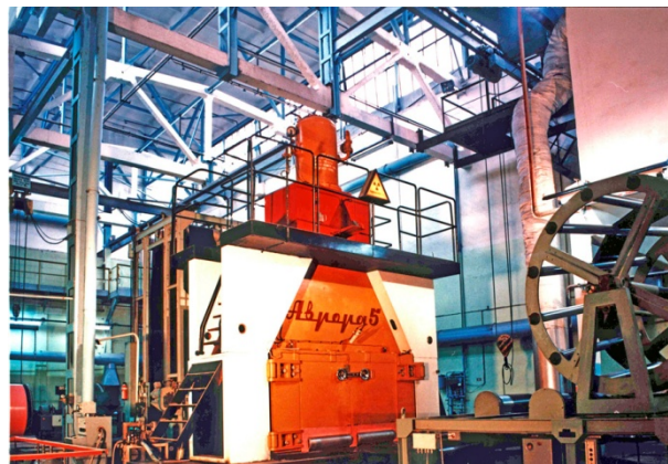
Figure 2: The “Aurora-5” accelerator in the line producing foamed polyethylene at the Izhevsk Plastic-Production Plant
