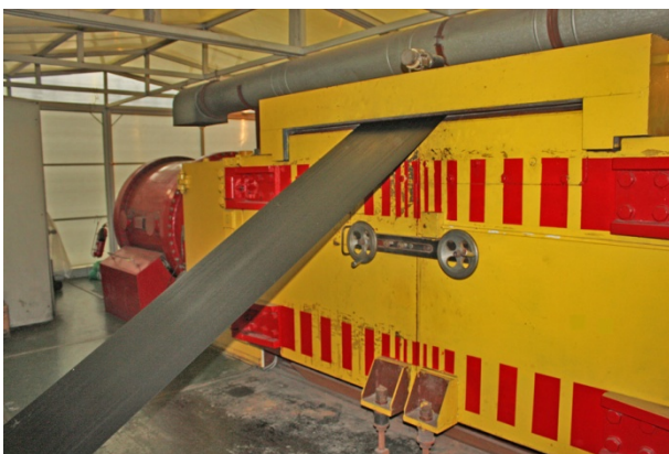
Figure 5: The “Electron-10” accelerator in the line for production of heat-shrinkage anti-corrosion coatings at the “IPM” Ltd, St. Petersburg
