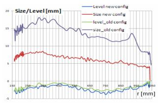
Figure 7: Parameters of the beam before and after correction of Q<sub>2</sub>-drop at 100mm
