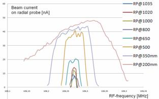
Figure 5: Smith & Garren curves at final configuration of the central plugs
