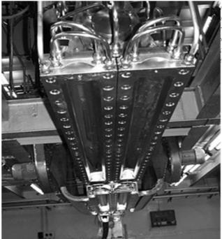
Figure 2. Double window extraction device of ELV-12 accelerator.
