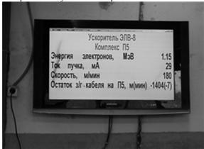
Figure 5. Parameters of accelerator ELV operation.
