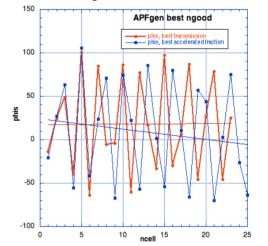
Fig. 3. The APF gap phase sequences for the best transmission (red) and best accelerated fraction (blue) cases. The linear fits show the effect of the tilt parameter.
