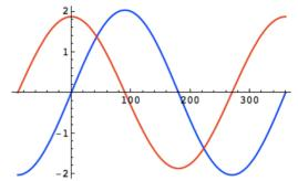
Fig. 1. Typical longitudinal acceleration (red) and transverse focusing forces (blue) over the full  $360^{\circ}$  range of phi.
