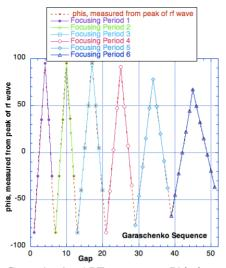
Fig. 2. Garaschenko APF sequence. Phis is measured from the peak of the wave. Overall the sequence is quasi-sinusoidal.
