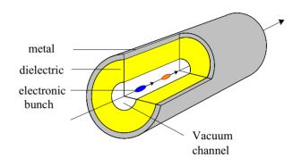
Figure 1: Wakefield waveguide structure.
