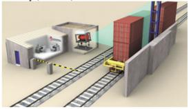
Figure 9: A rail cargo scanner.
