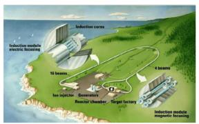
Figure 10: A conceptual view of a heavy ion inertial fusion power plant.
