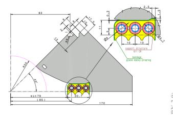
Figure 1: The 3-turn quadrupole magnet lamination design
