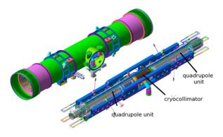
Figure 6: The doublet cryostat (above) and all the components mounted on the common girder.
