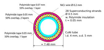
Figure 2: The cable of the corrector magnets.
