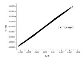
Figure 5: Distribution of particles in phase space y, y' on a channel B output.
