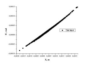
Figure 4: Distribution of particles in phase space x, x' on a channel B output.
