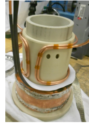
Figure 7: Discharge chamber with a short solenoid and new saddle antenna located out of solenoid.
