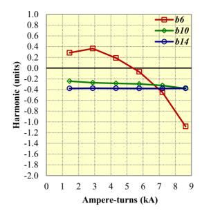
Figure 6: Measurements of harmonic terms dependence from current for quadrupole #9813-0001. Graphs show measurements for the same magnet with different nose pieces types: left – nose pieces have profile the same as yoke poles, right – nose pieces have **modified** profile.
