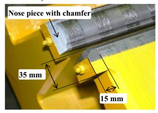
Figure 1: Nose pieces on one halve of magnet yoke.
