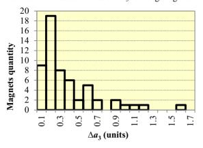
Figure 3: Statistic  $\Delta a_3$  in 65÷100 % of design current range for 60 long magnets.
