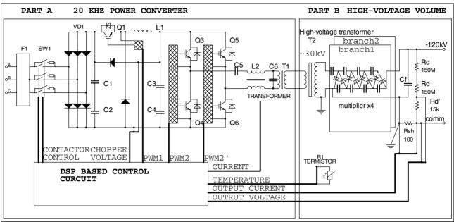
Fig.1. The high-voltage source block-diagram.
