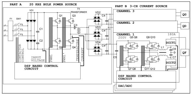
Fig.3. 3-channel current source circuit diagram.
