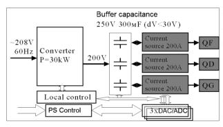
Fig. 2. Power source block diagram.
