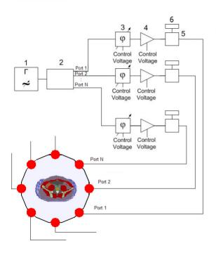
operate amplifiers and phase shifters. Signal from 1 generates a pulse-width modulation (PWM) signal. Further signal passing through RC-filters situated in both 2 and 3 units, goes to gate pin of amplifier. Because of control voltage of phase shifter varies in 0-12 V, we have to use operational amplifier with  $K_{\mu}=2.6$  in unit 3.
