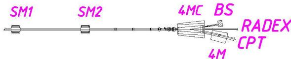
Figure 1: Layout of the beams separation: SM1, SM2 – steering magnets, 4MC – Lambertson magnet, 4M – bending magnet, BS – beam stopper, RADEX – neutron source, CPT – complex proton therapy.
