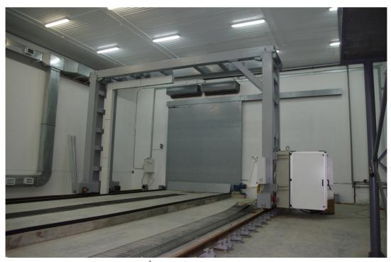
Figure 1: The IDK-6/9ÌeV accelerator in a customs inspection system.
