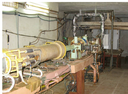
Figure 4: LINAC LUE-10 with conveyor and supercritical water convection loop.
