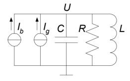
Figure 2: Equivalent circuit of the RF cavity.
