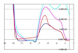
Figure 3: Dependence between the max real part of eigenvalues matrix M (vert.) and RF phases (hor.), calculated at the different detuning parameters ( $\xi$ =-1;-0.1;1;1000).
