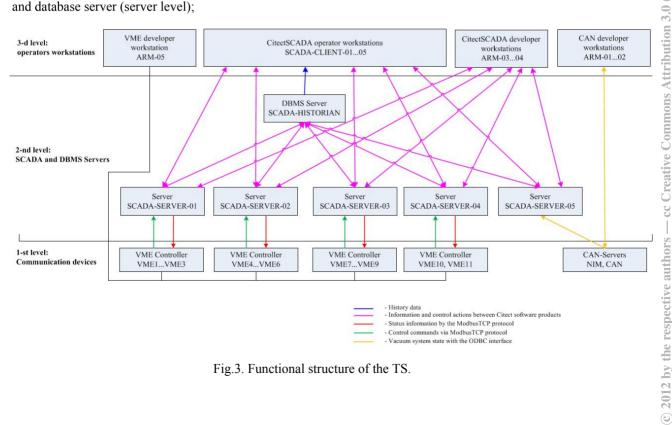
Fig.3. Functional structure of the TS.
