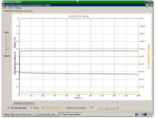
Figure 2: Circulation of the deuteron beam at the field plateau during 1000 s. Dipole field is 1.2 T (upper curve), the beam intensity is  $5 \cdot 10^9$  particles (lower curve). Blue curve – BCT signal in Volts. March 2012.
