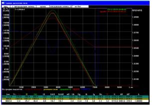
Figure 1: Cycle diagram at dipole magnetic field of 2 T. Red curve – basic function, yellow and green – field of the magnets and gradient of the lenses correspondingly. December 2010.
