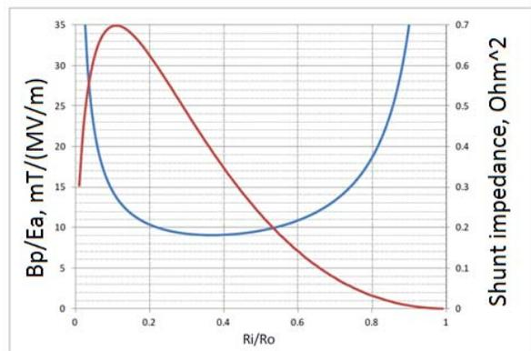
Figure 1:  $B_p/E_a$  and shunt impedance in QWR versus  $R_i/R_o$ .
