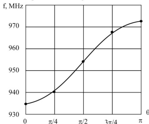
Figure 6: Dispersion curve for five cell elliptical accelerating cavity.
