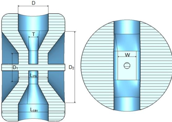
Figure 2: Cross-section of the spoke cavity with the geometrical parameters.
