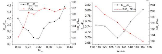
Figure 3:  $E_p/E_a$  (black) and  $R_a/Q_o$  (red) versus  $T/L_{iris}$  and  $W$ .
