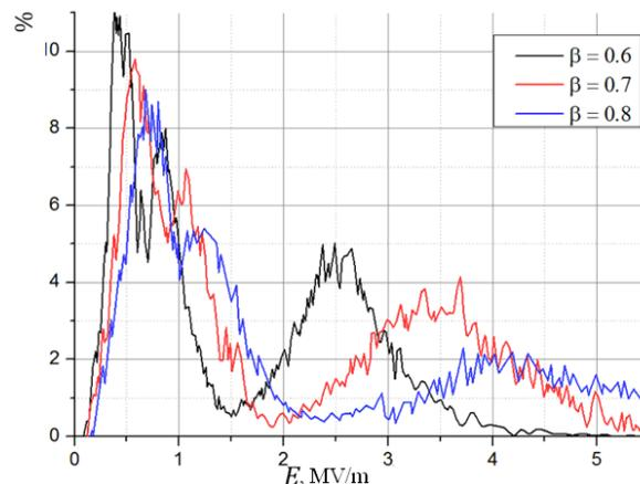
Figure 7: Particle number growth rate vs. field strength dependence
