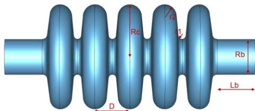
Figure 5: Five cell elliptical accelerating cavity.
