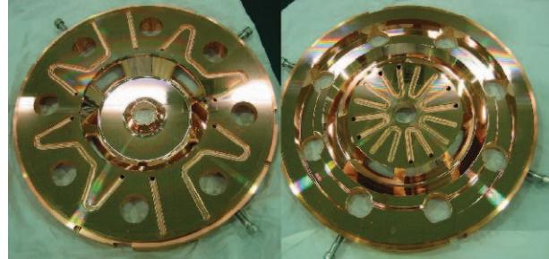
Figure 6: ACS half cells for J-PARC linac
