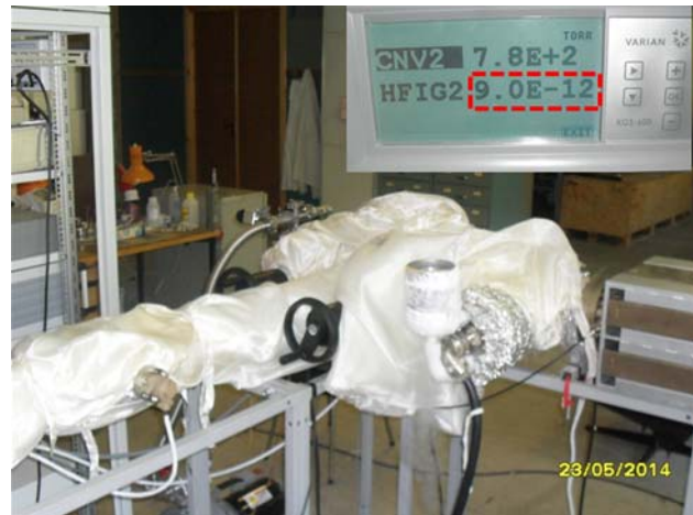
Figure 5: JINR vacuum test bench under the room temperature.
